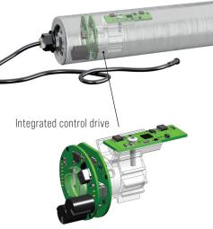
MTR 46 AD is today the most powerful motorized driven roller on the market, delivering 75W and 115W power ratings, enabling faster movement and higher payload capacity. Its advanced gearless direct drive design minimizes mechanical losses, reduces energy costs, and ensures quiet operation. The 48Vdc power supply enhances efficiency and simplifies wiring.
