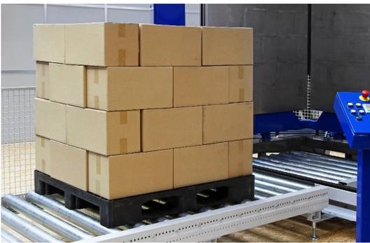
Pallet Conveyor allows efficient transport, accumulation, lifting and sorting of heavy loads as an alternative to forklifts handling. In warehouse automation operations a pallet conveyor is generally utilized to move loads of several hundreds kilograms while ensuring continuous feed of work and cutting edge efficiency. The high-performance synchronous brushless servomotor, coupled with planetary gearbox, ensures performance with loads up to 1500 kg per zone.
