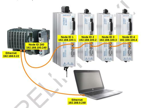
The X20 PLC operates as a Gateway between the standard Ethernet side (Laptop and IF2 on X20 PLC) and the Powerlink side (IF3 on X20 PLC and all drives). This enables the Metronix ServoCommander running on the laptop to reach the servo drives.
