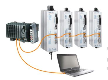
The single smartServo BL 4000 drives are connected in a line with the B&R X20 PLC. The Laptop, using B&R Automation Studio is connected to the connector IF2 of the X20 PLC. The first drive is connected to the IF3 connector (Powerlink) of the PLC via connector RTE0 of the drive.
