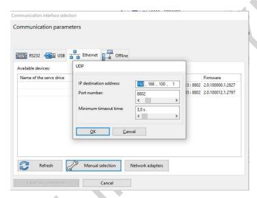
Press the "Manual selection" button in the "Communication interface selection" window to enter the desired IP address. The IP addresses of the individual nodes are composed of the fixed first 3 octets 192.168.100 and the node ID as the last octet. For example, the IP address for a CN with node ID 2 is 192.168.100.2.
