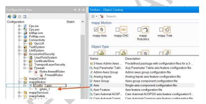
Finally, the smartServo BL 4000 must be configured as a "DS402-compliant drive" in Automation Studio. To do this, right-click on the drive icon in the physical view and open the "Configuration" dialog:
