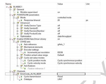
Especially the option "Enable DS402 Axis Driver Library" must be activated. Inside that option now the drive must be linked to the Axis instance that we just added in the "Configuration View" (in this example gAxis\_1). Encoder Settings should be set to 65536 increments per revolution.
