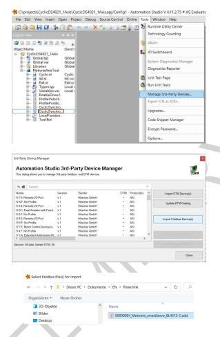
Afterwards the smartServo BL 4000 appears in the hardware catalogue of the Automation Studio and can be added to the hardware configuration of the project:
